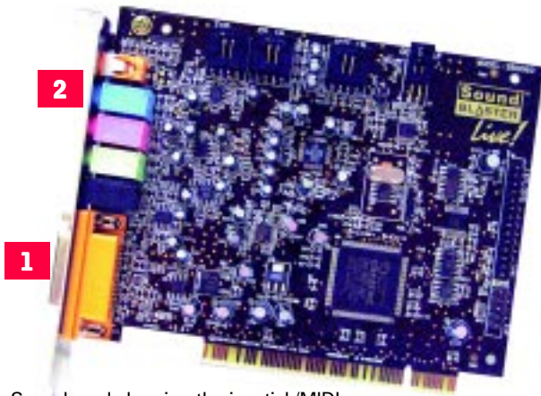
Sound card showing the joystick/MIDI connection [1], and 3.5 mm jack sockets [2]
